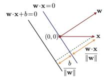
The geometric margin of h(x) on a set of examples  $T = \{x_1, ..., x_m\}$  is the minimal distance over these examples
